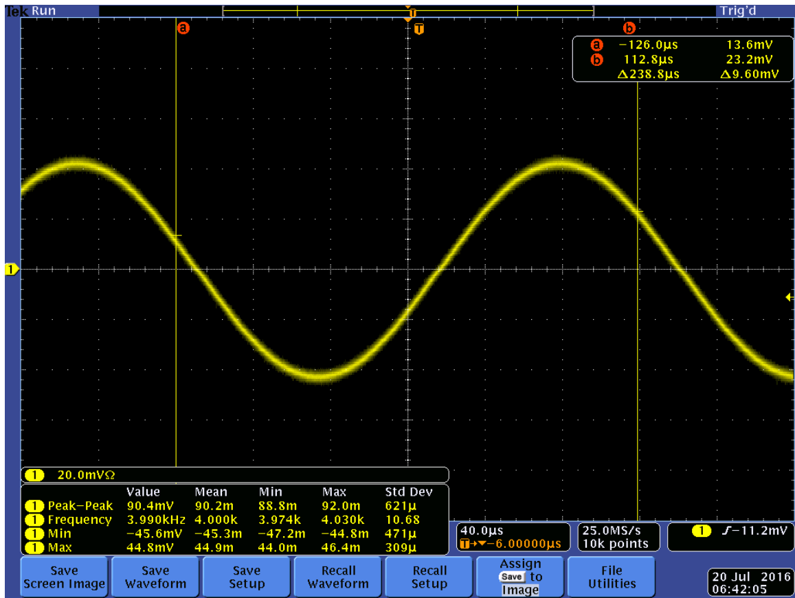
Figure 6.18 RX Audio Input with No Offset
